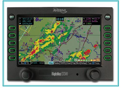
displays aviation weather at the highspeed update rates of the XM broadcast system, with the added benefit of the lower-cost, two-way datalink capability. *MultiLink* allows the operation of Avidyne's Narrowcast and XM's Broadcast weather individually or together as complementary systems, providing you with the best of both services.
