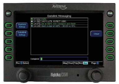
Avidyne's MultiLink two-way Text Messaging capability allows the pilot to send and receive messages between the EX500 and the Avidyne FlightCenter on the MyAvidyne.com website. Designated persons on the ground have the ability to send and receive text messages to and from the MultiLink-equipped aircraft, providing timely communication of such items as arrival time, itinerary changes, or flight plan deviations.
